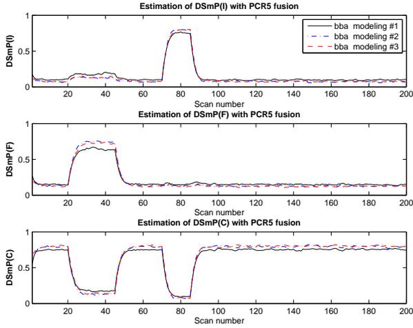
Figure 4.  $DSmP(.)$  results after using PCR5 rule of combination
