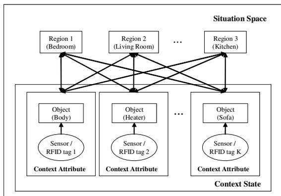
**Figure 1. A hierarchical interrelationships between sensors, related contexts, and relevant situation spaces based on a state-space modeling**
