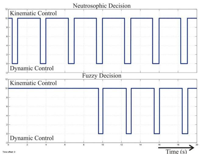
Fig. 8 Output data of the two switching techniques
