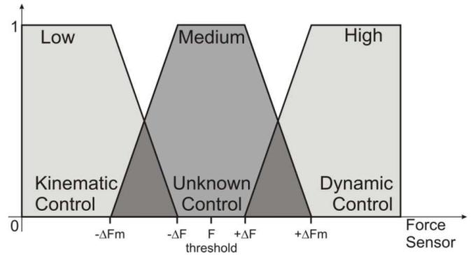
Fig. 3 Neutrosophication for the Force sensor data
