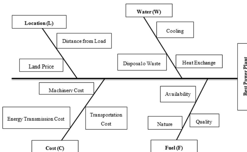
Figure 17. Fishbone diagram representing the necessities for setting up a power plant
